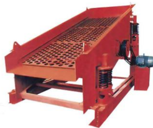
Secondary Screening Before Kiln (25mm)
