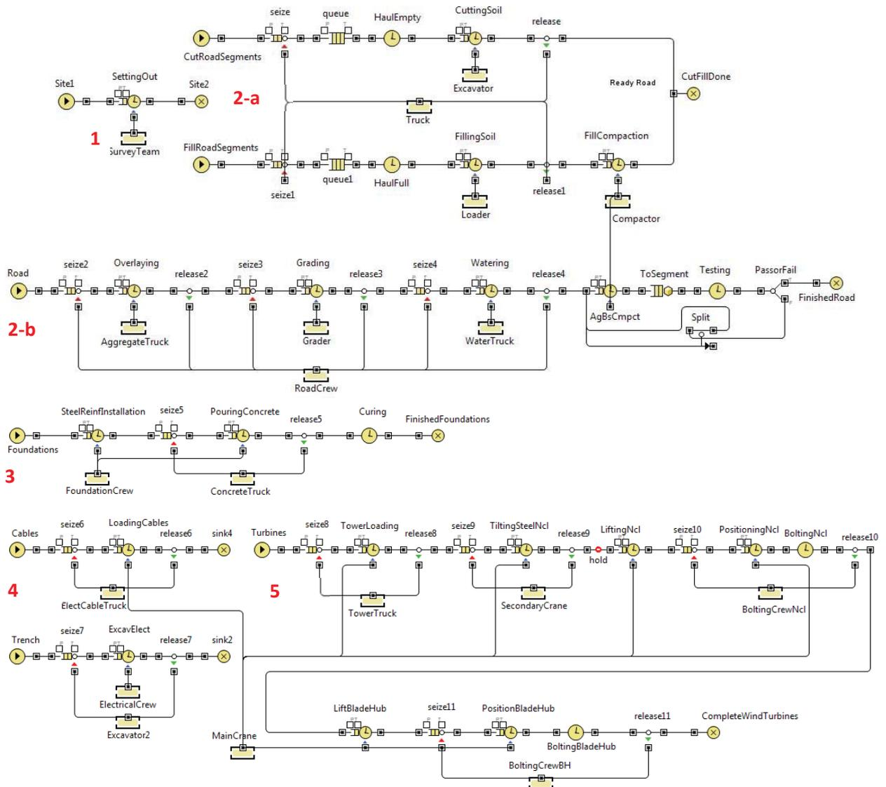
Figure 2. AnyLogic Model of the Construction Process
