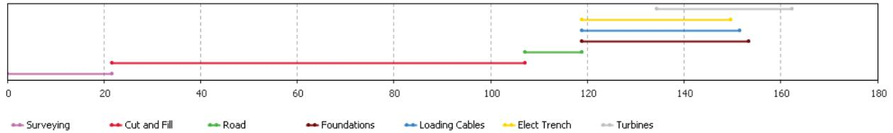
Figure 8. Optimized Gantt chart of the Falougha’s Wind Farm Construction Process (in working days)
